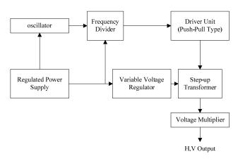
Fig. 1 Block diagram of high voltage unit
