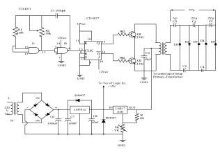
Fig. 6 Circuit diagram of the high voltage unit
