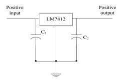
Fig. 4 Basic fixed-voltage regulator
