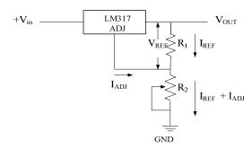
Fig. 5 Basic adjustable regulator using LM317IC
